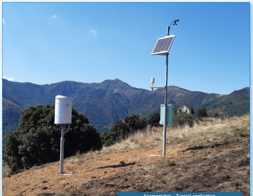
Anemometer - Typical application
